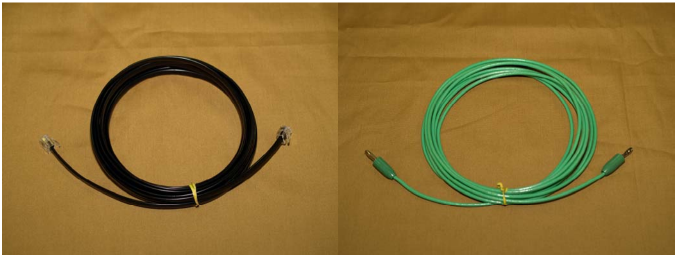
Figure 12 – Loconet and Ground Cables
