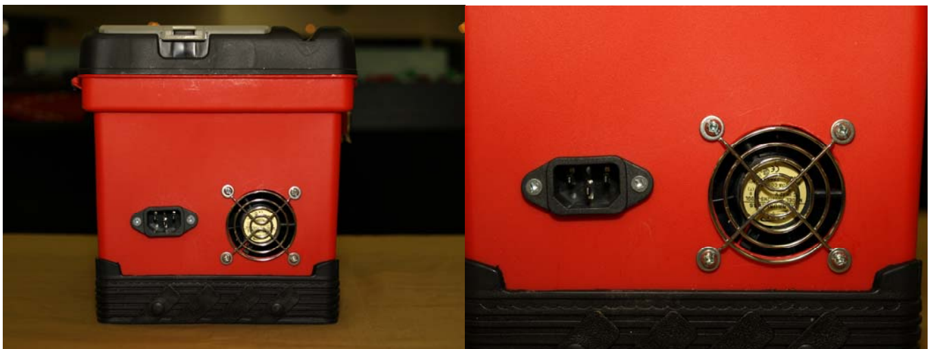
Figure 10 – Completed Input End Connections
