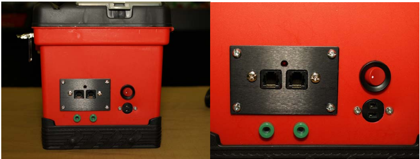
Figure 9 – Completed Output End Connections
